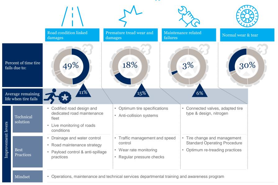
Note: Road condition linked damages include cuts, separation, sidewall damage, bead damage, tread damage and damage due to foreign objects. Premature tread wear and damages include premature wear and damage due to truck accidents. Maintenance related failures include repair failures and explosions
